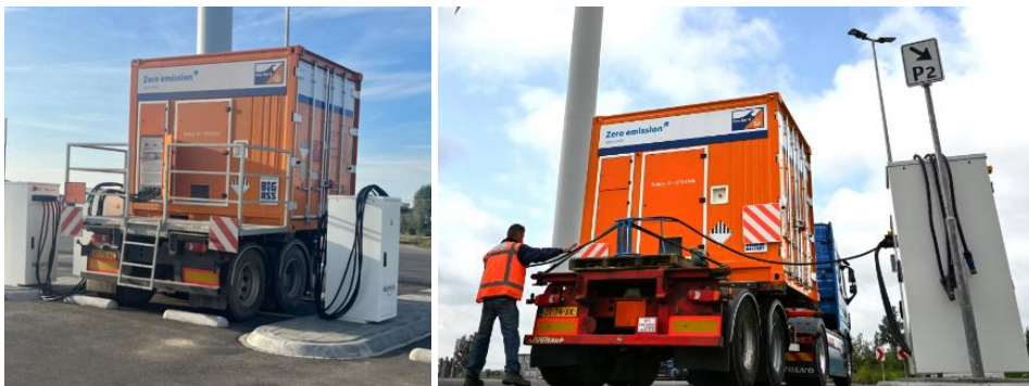
Figure 4.9: The container battery charging in the container charging area of WattHub. Connected to the AC charging (power lock) installation.
